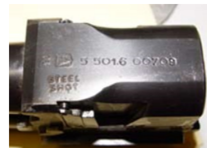
The underside of this over/under (o/u) shotgun breech shows it is suitable for steel shot cartridges.
