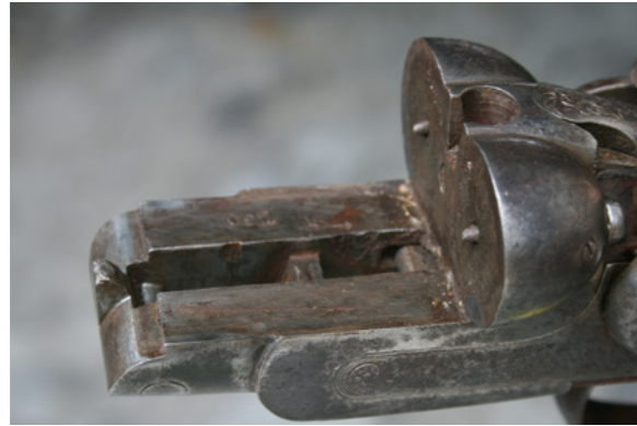
The firing pin (above) is stuck in the forwards position which means the gun may fire when closed. The force of the gun closing may cause the primer to detonate, resulting in an accidental discharge.
