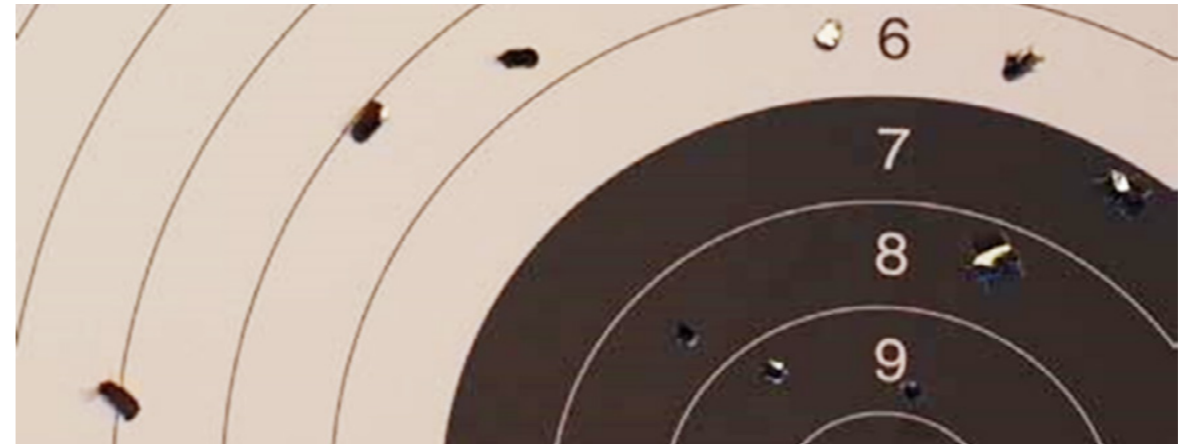
Projectiles that have not stabilised will flip over during flight.
