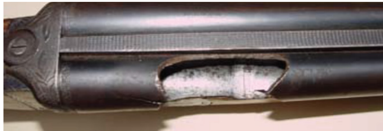
The 12 gauge side-by-side shotgun above was destroyed by firing into a barrel that had been blocked by a wad from a previous faulty cartridge.
