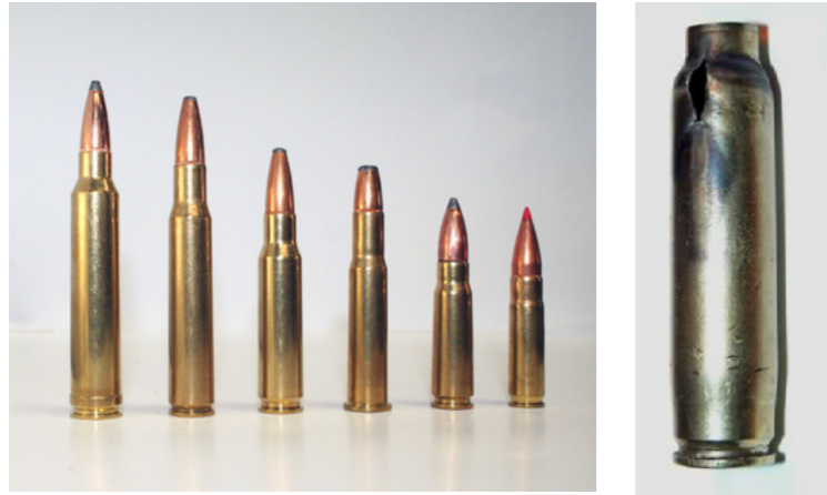
Cartridges from left to right: .300 win mag, 30/06 Springfield, .308 Winchester, 30-30 Winchester, 7.62 x 39 Russian, .300 Blackout. Far right: Effects of a 7.62 x 39 being fired from a .308 Winchester.
