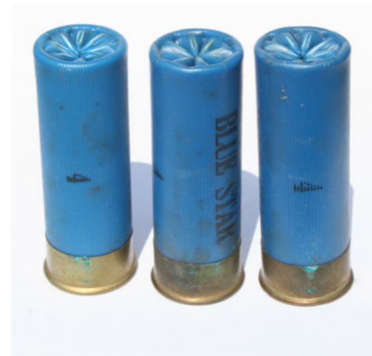
Storing ammunition in a damp environment may cause corrosion.
