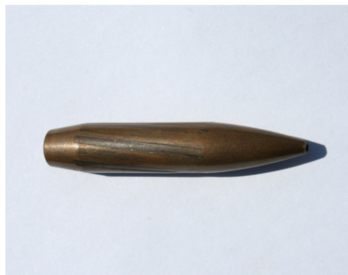
Rifling marks left on a projectile.
