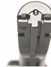
The firing pin of an uncocked rimfire rifle (above). Note the protruding firing pin.
