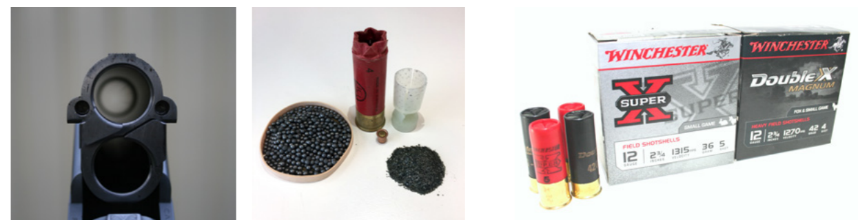
Smooth bore of a shotgun (above left). Components of a shotgun cartridge including case, powder, primer, propellant, wad and shot (above centre). Factory shotgun ammunition (above right).
